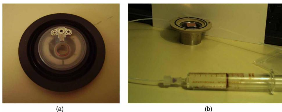
**Fig. 6** (a) Upper half of the fluid cell, with the black Viton™ membrane; and (b) lower half of the fluid cell with the new aluminium part and a syringe with solvent attached to the Luer fittings
