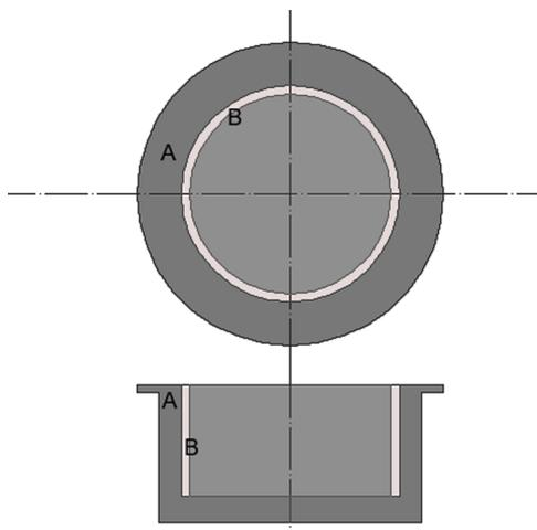
**Fig. 2** Container pot of the modified AFM closed fluid cell for tribological investigations of large samples in chemically aggressive environments, top and side view
