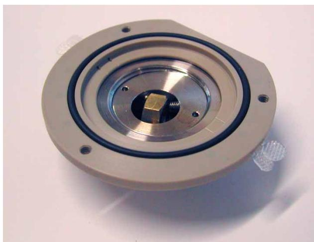
**Fig. 5** Assembled modified AFM closed fluid cell for tribological investigations of large samples in chemically aggressive environments. The sample is an M4 brass screw nut, 1 cm in diameter, 5 mm high
