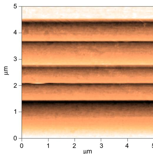
**Fig. 11** *In situ* AFM scan. The stripes appear when the heptan + ZDDP solution is introduced into the fluid cell, because the tip intermittently loses connection with the sample
