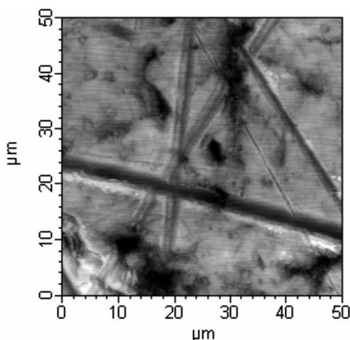
**Fig. 10** AFM intermittent contact mode image in toluene of wear marks on 100 Cr6 steel in the open-cell configuration. Image size  $50 \times 50 \mu\text{m}^2$
