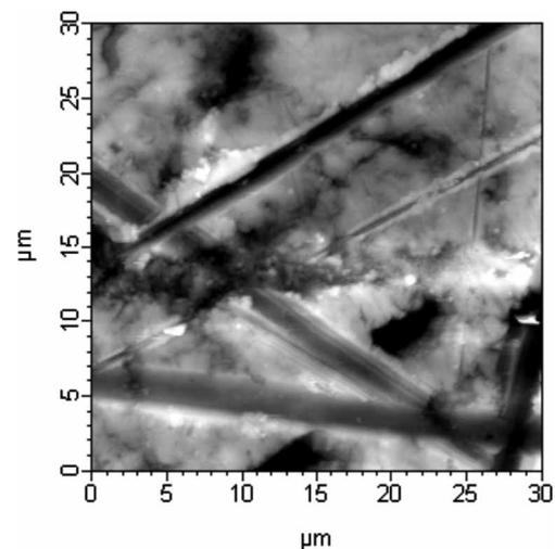
**Fig. 8** AFM contact mode image in toluene of wear marks on 100 Cr6 steel in the open-cell configuration. Image size 30×30 μm<sup>2</sup>
