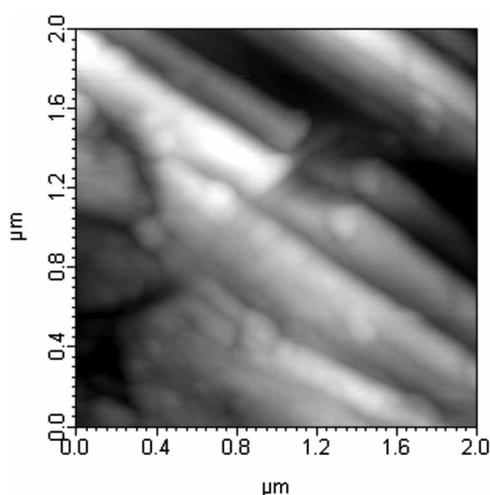
**Fig. 9** AFM contact mode image in toluene of wear marks on 100 Cr6 steel in the open-cell configuration. Image size  $2 \times 2 \mu\text{m}^2$
