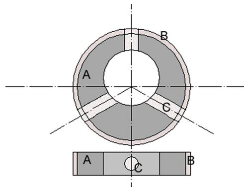
**Fig. 3** Sample holder for the modified AFM closed fluid cell for tribological investigations of large samples in chemically aggressive environments, top and side view
