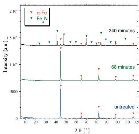
Fig. 7: XRD-patterns of thermochemically treated steel substrates with different nitriding times. bottom: polished substrate; middle: 68 minutes; top: interruption after 240 minutes (compound layer: Fe<sub>4</sub>N)
