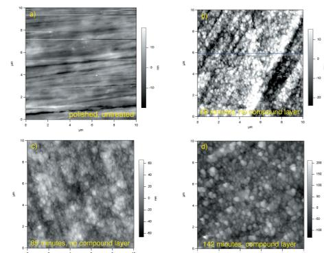
Fig. 6: AFM-images of the surface morphology of nitrided steel substrates with different nitriding times. a) untreated; b) 68 minutes; c) 85 minutes; d) 142 minutes (with compound layer)
