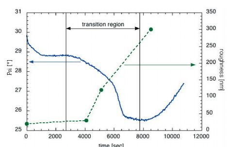
Fig. 7: Relationship between the  $\Psi$  signal and the roughness obtained from AFM measurements.
