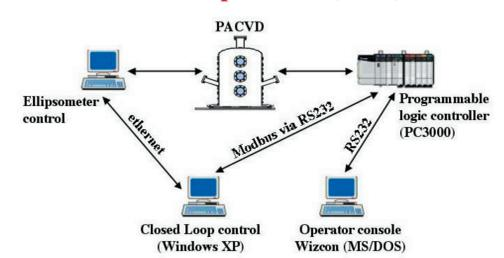
Fig. 9: Computer network of the closed loop control system.
