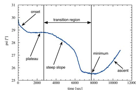
Fig. 3: Kinetic measurement of  $\Psi$  during the nitriding step.
