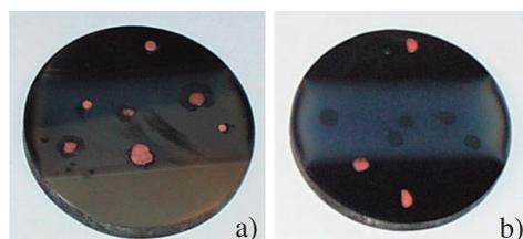
Fig. 4: Redox reaction of copper sulphate solution with treated substrates.
