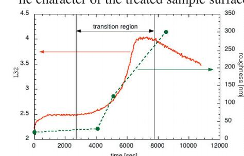
Fig. 10: (Proportional-integral) PI-control of the nitriding step with the average value and the setpoint. The PI-controller starts to regulate the process when the setpoint is passed by the control variable L<sub>32</sub> for the first time in order to avoid compound layer formation.
