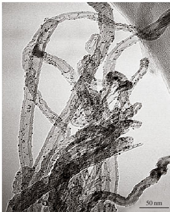
**Fig. 3.30** Transmission electron microscopy image showing rhodium nanoparticles supported on MWNT surface (from [3.235])
