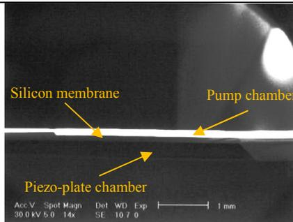
Fig. 7. Cross-section view of fabricated membrane after double sided silicon etching
