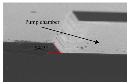
Fig. 6. The fabricated pump chamber with 54.7° wall side slope and clean surface.
