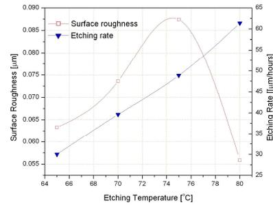
Fig. 4. Surface roughness and etching rate at various temperature
