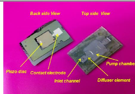
Fig 8. Photograph of fabricated pump at back side and front side
