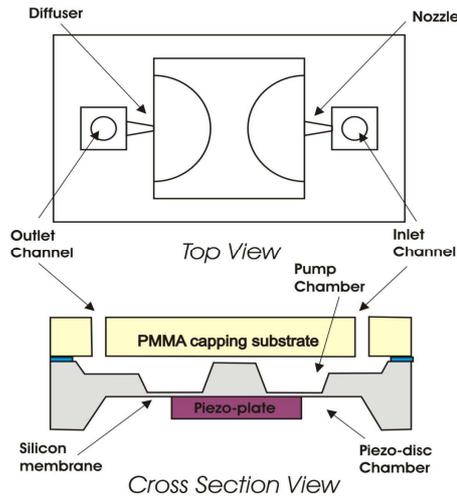
Fig. 1. Schematic design of PVLMP (Planar Valveless Micropump)
