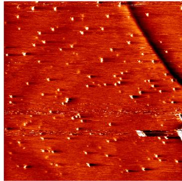
Figure 2:  $Ar^{16+}$  different sized hillocks; image size  $200 \times 200 nm^2$ ; current image
