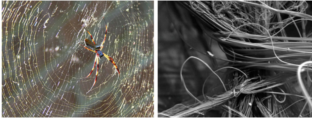
Fig. 12 Spider silk is a strong and lightweight material. Its functionality is based on properties emerging from smart arrangement of perfect nanocrystals within a soft matrix and further levels of hierarchy at various length scales
