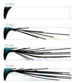
Simulation of charging effects in insulating capillaries taken from ref. [3].
