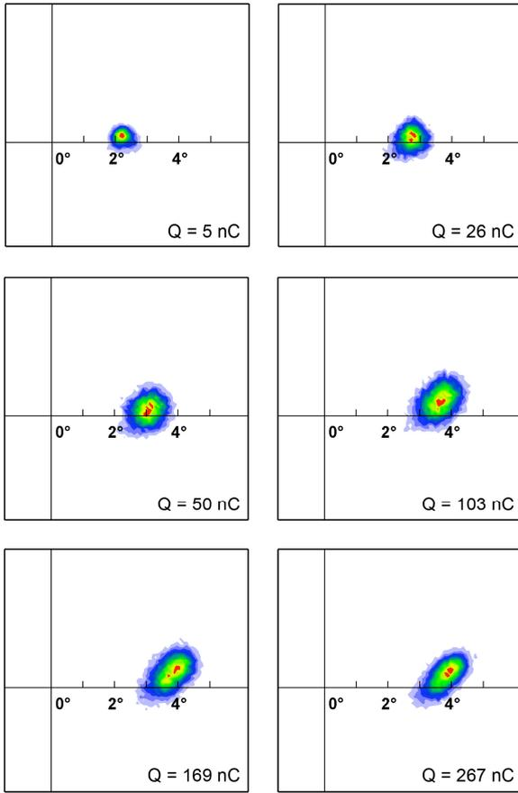
**Figure 2.** Evolution of the measured 2-dim. scattering distribution for 12 keV  $\text{Ar}^{8+}$  ions transmitted through PET capillaries (tilt angle  $4^\circ$  with respect to the incident ion beam direction) during the charging-up phase.  $0^\circ$  corresponds to the position of the incident ion beam (i.e. when removing the nano-capillary target).
