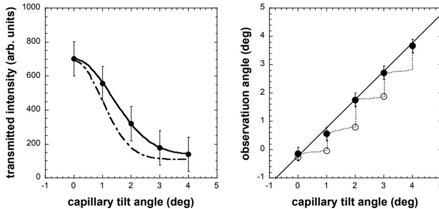
**Figure 1.** Intensity of the transmitted projectiles (left) and observed peak angle of "guided" projectiles (right) after transmission of the PET capillary target as a function of capillary tilt angle for 12 keV  $\text{Ar}^{8+}$  projectiles (c.f. text).
