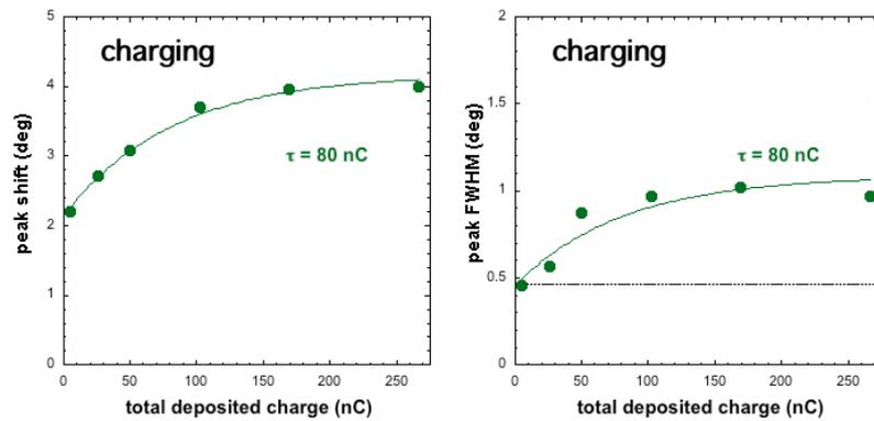
**Figure 3.** Peak position and width of the guided projectiles as a function of total deposited charge during the charging-up phase. Data for 12 keV  $\text{Ar}^{8+}$  projectiles and  $4^\circ$  tilt angle.
