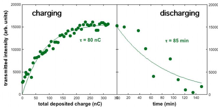
**Figure 4.** Evolution of the transmitted intensity as a function of total deposited charge during the charging-up phase (left) and as a function of time during the discharging phase (right). Data for 12 keV Ar<sup>8+</sup> projectiles and 4° tilt angle.
