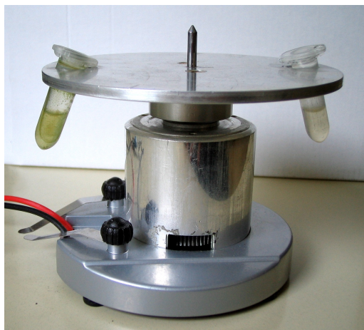
Figure 6: Centrifuge designed by Clemens Grünberger.
