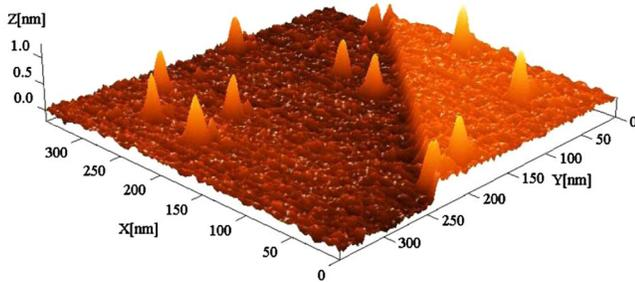
FIG. 1 (color online). Topographic contact-mode AFM image of a  $\text{CaF}_2(111)$  surface after irradiation with  $2q$  keV  $\text{Xe}^{33+}$  ions showing hillocklike nanostructures protruding from the surface.
