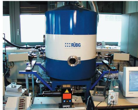
Fig. 1: The adapted PACVD reactor and the experimental setup of the in-situ ellipsometer.
