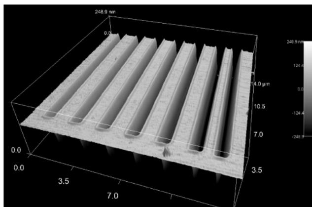
**Figure 1:** Silicon Chip with Defined Slots Prepared by FIB
