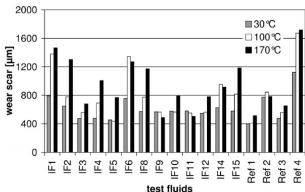
Figure 3: Wear Behaviour of Ionic Liquids and Reference Oils at 30, 100 and 170 °C
