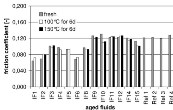
Figure 6: Friction Behaviour of Ionic Liquids and Reference Oils Aged at 100 and 150 °C
