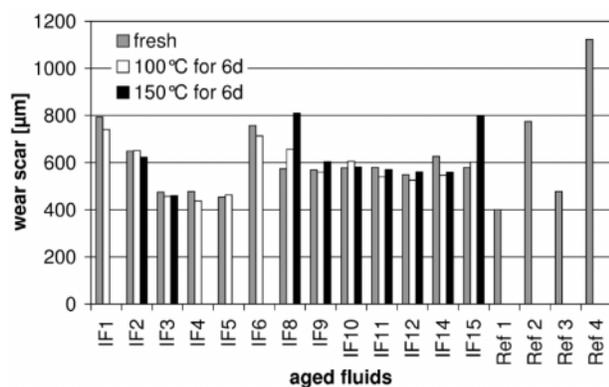
Figure 5: Wear Behaviour of Ionic Liquids and Reference Oils Aged at 100 and 150 °C
