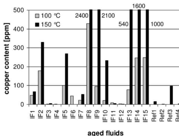
**Figure 2:** Copper Content in Ionic Liquids and Reference Oils after Artificial Ageing
