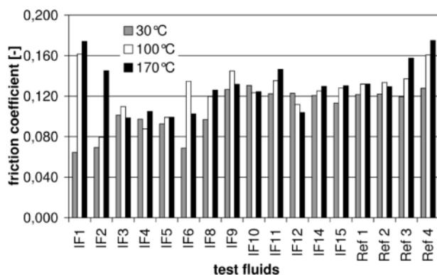
Figure 4: Friction Behaviour of Ionic Liquids and Reference Oils at 30, 100 and 170 °C
