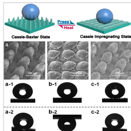
Fig.2 Changes in surface morphology during the compressing/recovering process and their related shape of water droplets on the surfaces: static water contact angles ( $a_1$ ,  $b_1$  and  $c_1$ ), roll-off angles ( $a_2$ ,  $b_2$  and  $c_2$ ).
