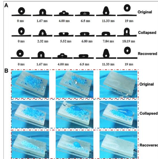
Fig.3 A) Drop dynamical impacting behaviours displayed by the selected snapshots of a droplet vertically impacting on horizontal surfaces. B) Self-cleaning process on the sample surfaces with a  $15^\circ$  tilting angle.
