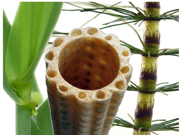
*Fig. 3: The Technical Plant Stem (center) an ultra-lightweight fibrous compound structure with two of its biological models giant reed (left) and horsetail (right) © PBG Freiburg & ITV Denkendorf*
