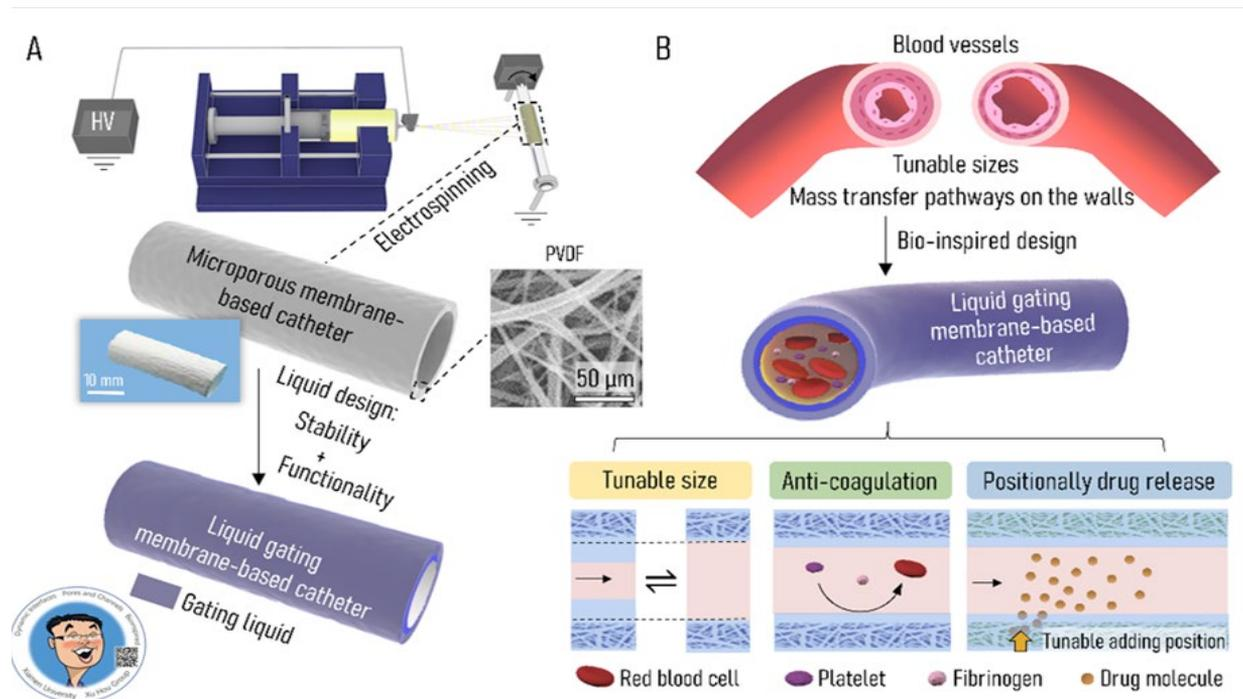
Fig. 1. Design and preparation of bio-inspired liquid gating membrane-based catheter
