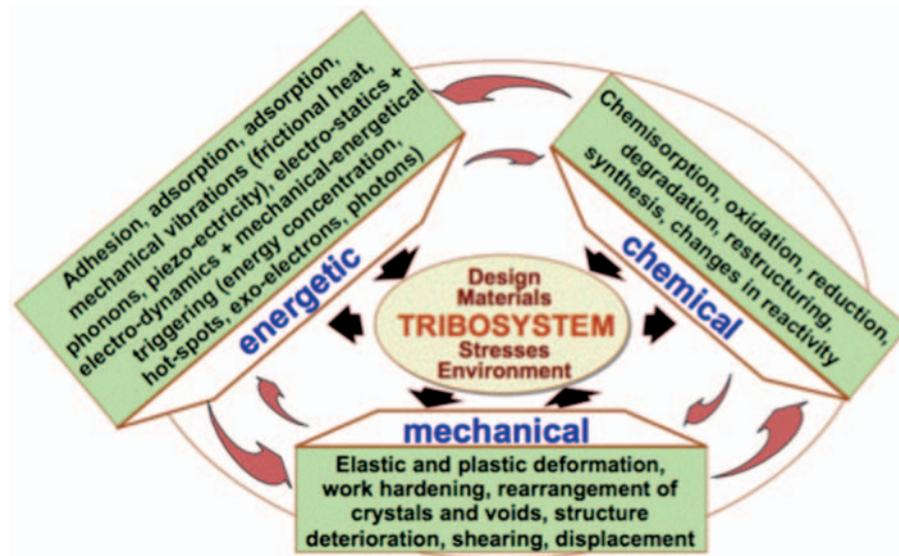
**Fig. 6** Effects and their causes in a tribological system – the tribological triangle. © F. Franek, Austrian Center of Competence for Tribology, using the tribological triangle concept from H. Faigle, Faigle Kunststoffe, Austria. <http://www.faigle.com>. Image reproduced with permission
