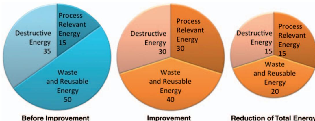
**Fig. 3** Tribosystem optimization (estimated values, may vary depending on process). (a) Before improvement. (b) Step 1: improvement of share of process-relevant energy and reduction of non-relevant energy share. (c) Step 2: reduction of total energy required for same output. Note that the destructive energy and the waste and reusable energy portion are less than half compared to the respective values in the initial tribosystem in Fig. 3(a)
