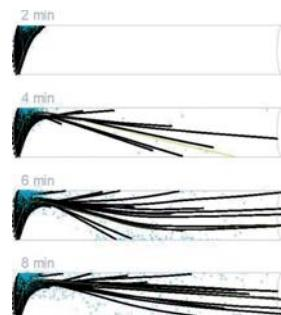
Simulation of charging effects in insulating capillaries taken from ref. [3].
