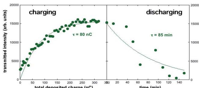
Evolution of the transmitted intensity as a function of total deposited charge during the charging-up phase (left) and as a function of time during the discharging phase (right). Data for 12 keV  $\text{Ar}^{8+}$  projectiles and  $4^\circ$  tilt angle.
