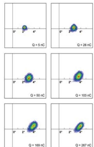
above: Image of the "direct beam".  $0^\circ$  corresponds to the position of the incident ion beam (i.e. when removing the nano-capillary target).
