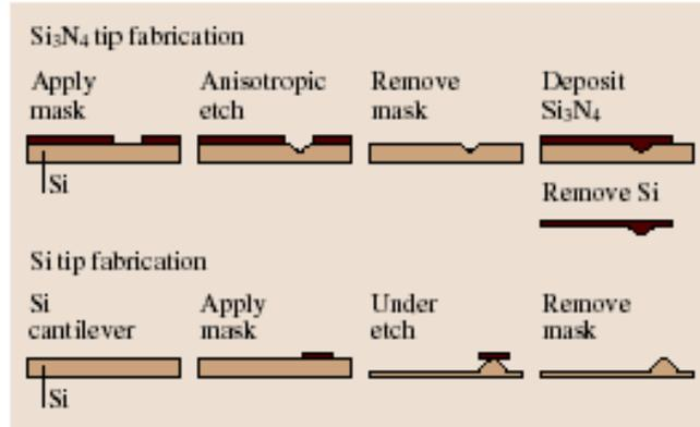
**Figure 11: Tip fabrication technique[14]**
