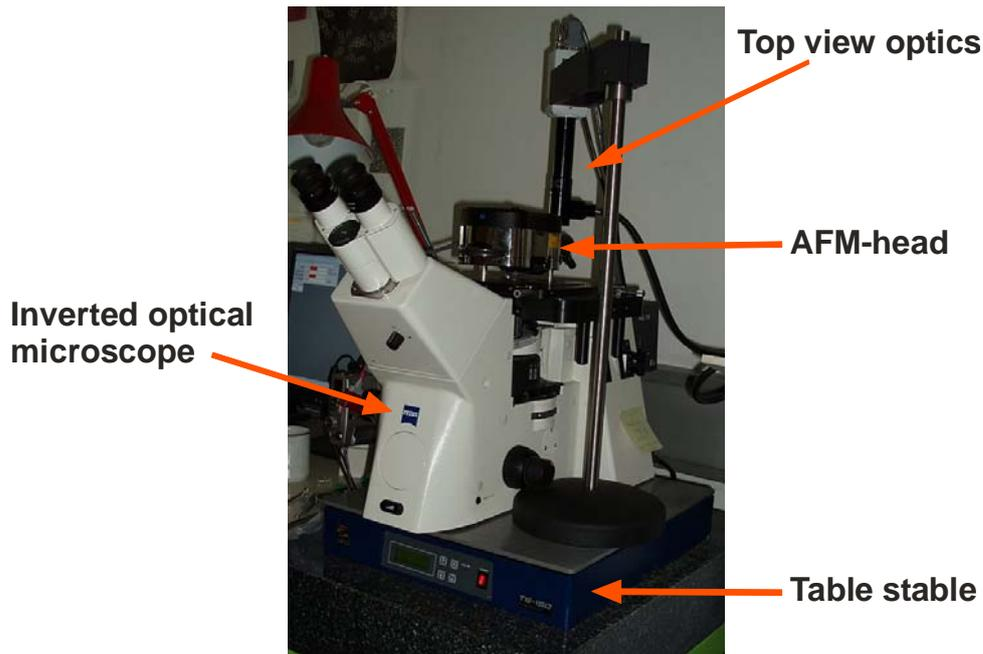
Figure 9: AFM and its components (MFP3D-Asylum Research).
