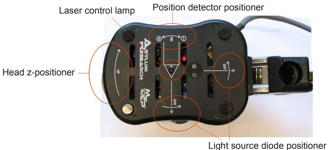
**Figure 29: AFM head explanation.**
