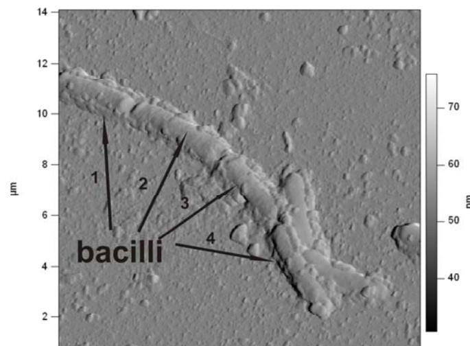
Figure 6: Chain of four vegetative *Bacilli subtilis*, Amplitude Trace, scan size 14 $\mu\text{m}$  x 14 $\mu\text{m}$ .
