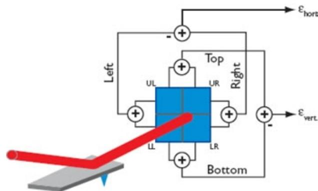
Figure 13: Diagram of a position sensitive detector.
