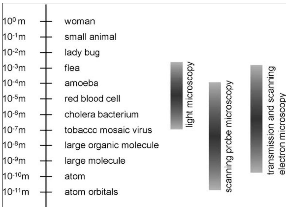
Figure 2: Scaling of the microcosms and the relevant microscopically techniques[5].
