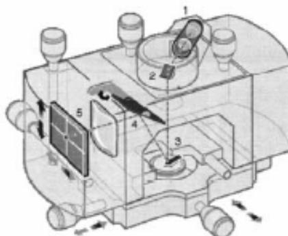
Figure 10: Inside of the AFM head. 1) Laser; 2) Mirror; 3) Cantilever; 4) Mirror; 5) Detector.
