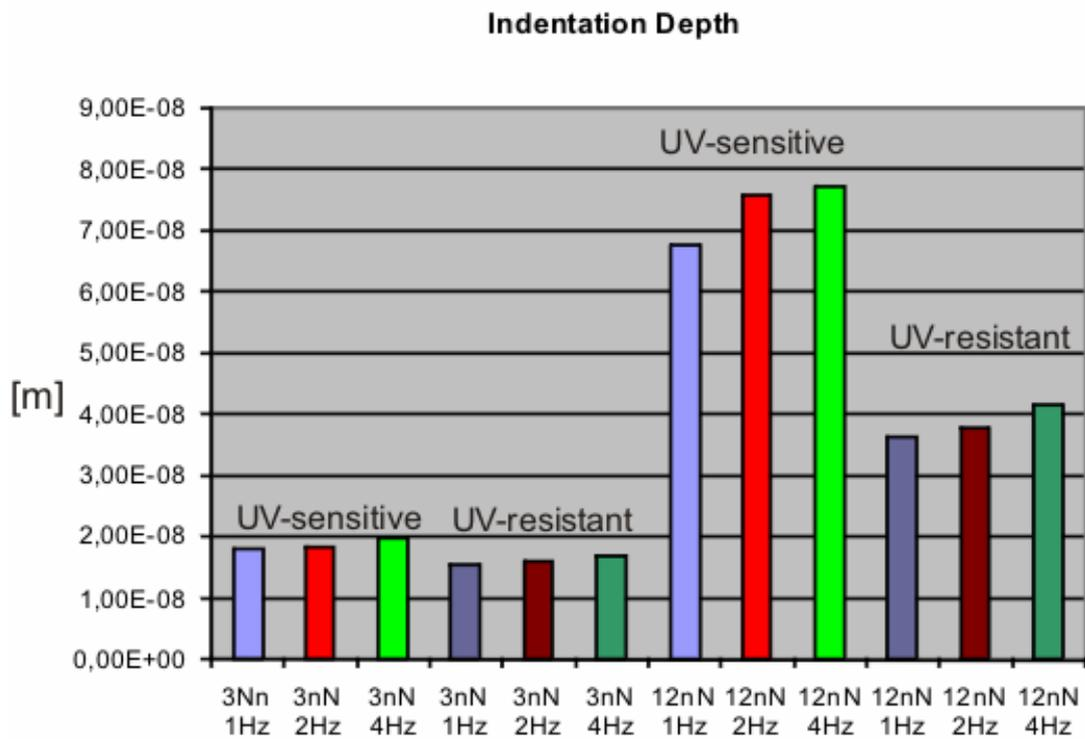
**Figure 47: Diagram of the difference of the indentation depth of UV-sensitive and UV-resistant *Bacillus subtilis* spores at different indentation forces and speeds.**
