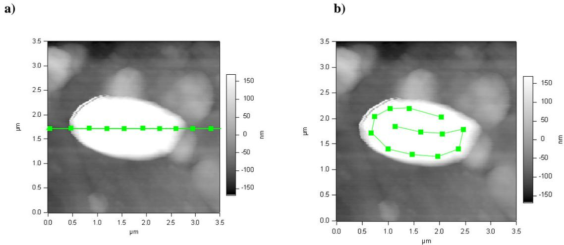
**Figure 33: Force mapping of *Bacillus subtilis* spores: a) Force mapping points given on a line; b) Force mapping points arranged on a user-defined path.**
