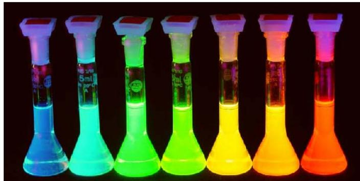
**Figure 4: Fluorescence induced by UV-radiation of different sized CdSe quantum dots[10]. They confine the charge carrier in all three spatial directions, so that the spectrum is discrete depending on their size.**
