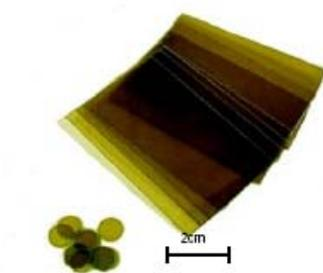
Figure 21: Samples of Mica structure for AFM measurements.
