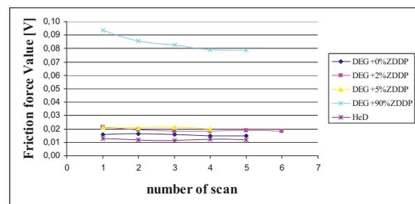
Figure 7: Friction force value vs. number of scans for a set point of 5V and a scan speed of 12  $\mu\text{m/s}$ .
