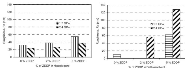
Figure 2: Comparison of roughness after the tribo tests.
