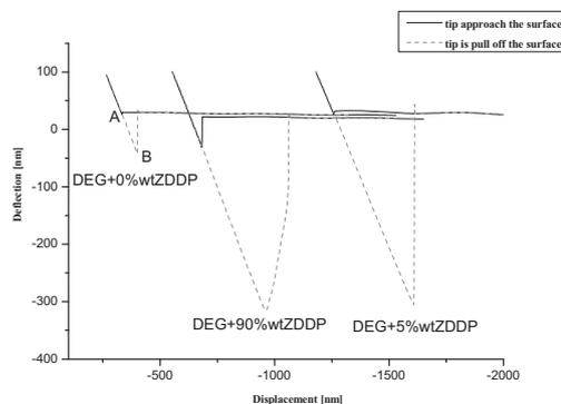
Figure 3: Pull of force curves of investigated samples.
