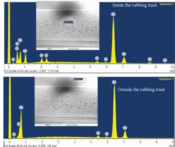
Figure 1: EDS spectra and SEM images inside and outside the running track of specimen tested with DEG + 2% wt ZDDP.
