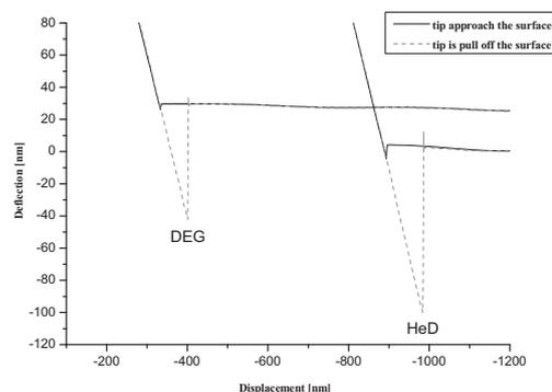
Figure 4: Pull of force curves of surface with DEG and HeD oil.
