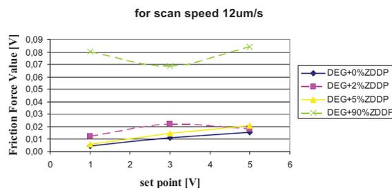
Figure 5: Friction force value vs. set point for a scanning speed of 12 μm/s.
