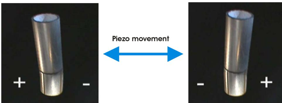
Figure 16: Movement of the piezo tube in x and y direction[47].
