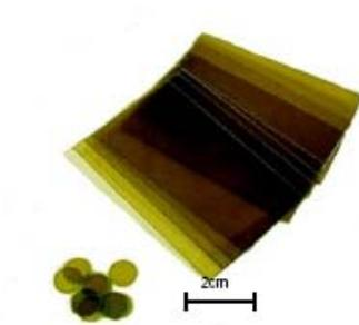
Figure 21: Samples of Mica structure for AFM measurements.
