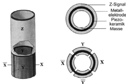
Figure 15: Schematic view of a four segment piezo tube[44].
