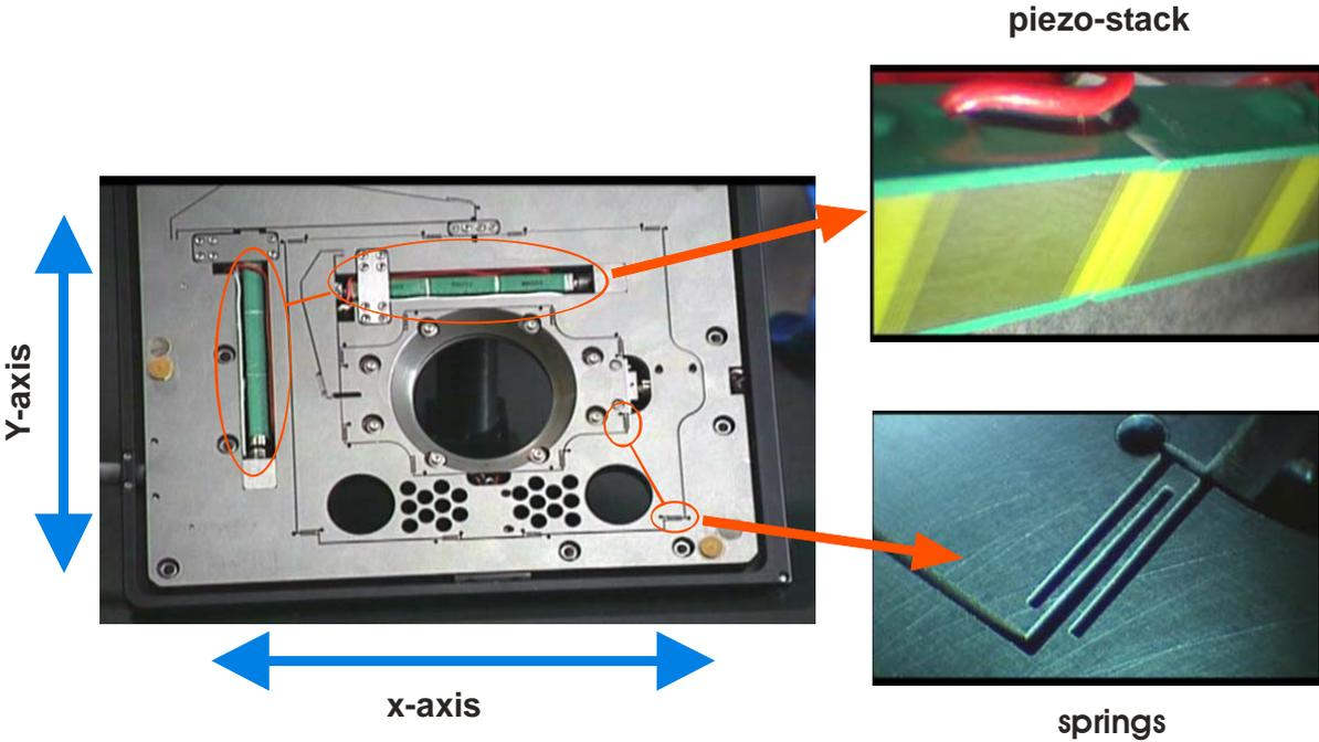
Figure 17: Bottom view of the central stage.
