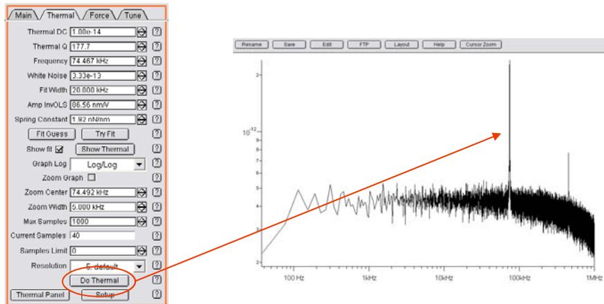
**Figure 30: Thermal Tune, yielding the resonance frequency of the cantilever.**
