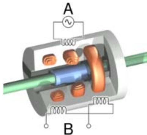
Figure 18: Cutaway view of a LVDT.
