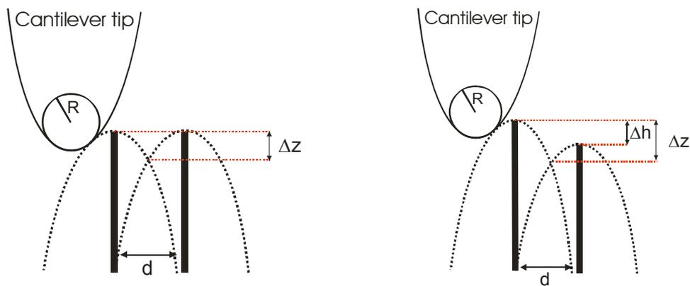
Figure 19: Resolution depending on the tip shape of a cantilever.
