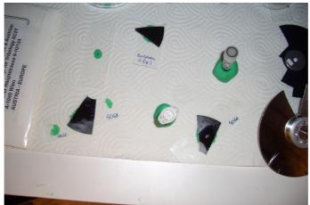
figure 1: 40 GB sample for MFM meassurements
