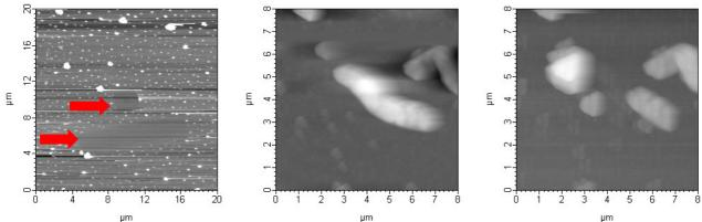
figure 12: scratched areas on gold figure 13: bacteria before scratch surface
