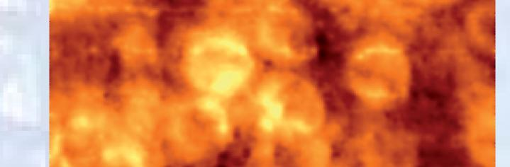
400 nm square, sample bias +1.5 V, 0.2 nA tunnelling current, 5x10<sup>10</sup> impacts per square cm with other parameters as in the image to the left before oxidation. The profiles of the apparent impact sites is essentially similar to those seen in the other picture and the number density is consistent with the increased dose; a raised area about 50 nm in diameter with a fairly flat top. More analysis has not been carried out; the image was collected last Thursday!
