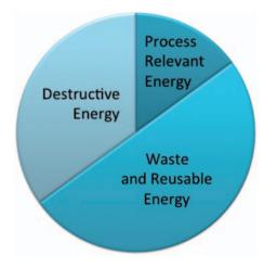
**Fig. 2** Energy distribution in a typical tribosystem with room for improvement. The process-relevant energy is just a small portion of the total energy, i.e. destructive and waste and reusable energy have a dominant share
