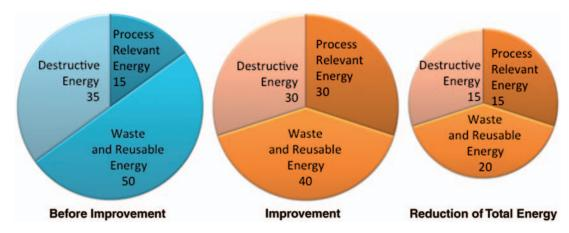
**Fig. 3** Tribosystem optimization (estimated values, may vary depending on process). (a) Before improvement. (b) Step 1: improvement of share of process-relevant energy and reduction of non-relevant energy share. (c) Step 2: reduction of total energy required for same output. Note that the destructive energy and the waste and reusable energy portion are less than half compared to the respective values in the initial tribosystem in **Fig. 3**(a)
