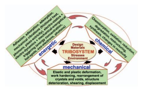
**Fig. 6** Effects and their causes in a tribological system – the tribological triangle. © F. Franek, Austrian Center of Competence for Tribology, using the tribological triangle concept from H. Faigle, Faigle Kunststoffe, Austria. http://www.faigle.com. Image reproduced with permission
