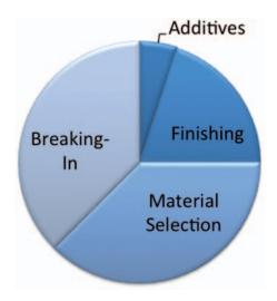
Fig. 4 Optimization levers in tribology.  $\bigcirc$  2010 M. Scherge,  $\mu$ CT Microtribology Center Karlsruhe. Image reproduced with permission
