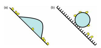
**Fig. 5** Schematic diagram: (a) on a conventional flat surface, the liquid droplet slides over the dirt and only redistributes the particles; (b) on a self-cleaning surface, the dirt particles have only small contact area with the surface, and the large contact angle of the liquid droplet causes the droplet to roll over the surface, with the dirt particles adhering to the droplet
