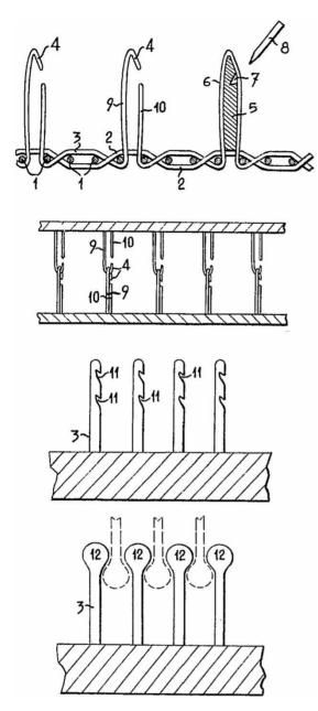
**Fig. 4** Drawings from the 1951 patent application for a 'Velvet type fabric and method of producing same' showing different possibilities for reversible attachment systems. Source: http://v3. espacenet.com/origdoc?DB=EPODOC&IDX= CH295638&F=0&QPN=CH295638
