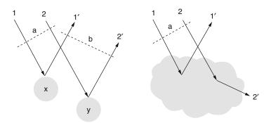
Fig. 4 Coherent (left) and incoherent scattering (right)
