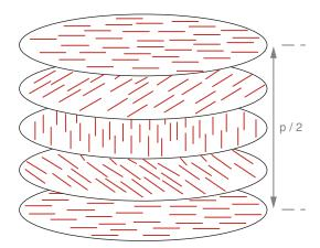
**Fig. 6** The chiral nematic phase in a cholesteric liquid crystal. *p* refers to the chiral pitch (Image reproduced with permission under the terms of the GNU Free Documentation License)
