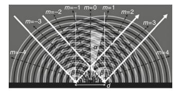
Fig. 3 Schematic of the color generating mechanism by the diffraction of light by a diffraction grating (black bar on bottom)
