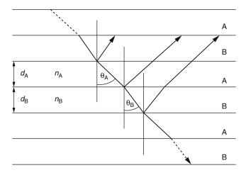
Fig. 2 Multilayer interference.  $n_{\rm B} > n_{\rm A}$ . A change in viewing angle corresponds to a change in the perceived color, due to changes in the apparent film thickness
