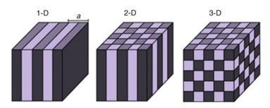
**Fig. 5** Schematics of one-, two-, and three-dimensional photonic crystals (1-D, 2-D, 3-D). The colors represent materials with different refractive indices. The spatial period of the material is called the lattice constant, *a*
