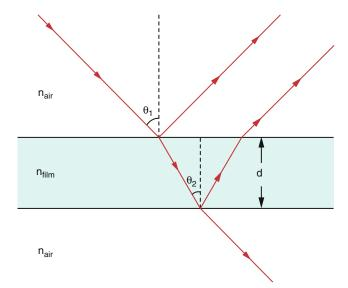
Fig. 1 Thin-film interference in the case of, for example, soap bubbles
