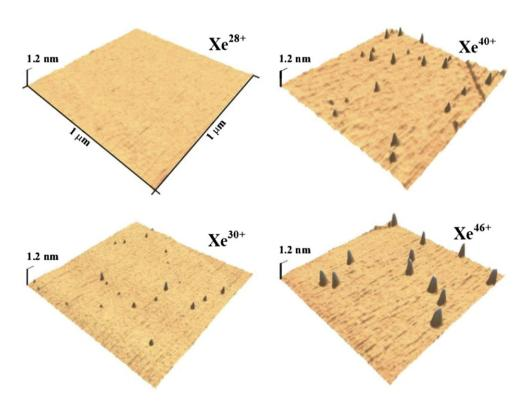
Fig. 1. Topographic contact-mode AFM images of a CaF<sub>2</sub>(111) surface irradiated by 10q keV  $Xe^{q^+}$  ions of charge state q=28, 30, 40, 46. In each frame an area of  $1 \mu m \times 1 \mu m$  is displayed. Hillock-like nanostructures protruding from the surface are only observed for Xe projectiles with charge state  $q \ge 30$ . Above this threshold, the height and diameter of the hillocks increase with ion charge state.
