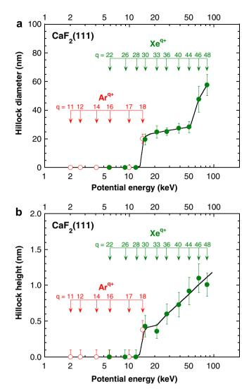
Fig. 2. Mean diameter (top) and height (bottom) of hillock-like nanostructures as a function of the potential energy of  $Ar^{q+}$  (open symbol) and  $Xe^{q+}$  (full symbol) projectiles. Hillocks are found only above a potential energy threshold of about 14 keV. The error bars correspond to the standard deviation of the diameter and height distributions; the solid lines are drawn to guide the eye.
