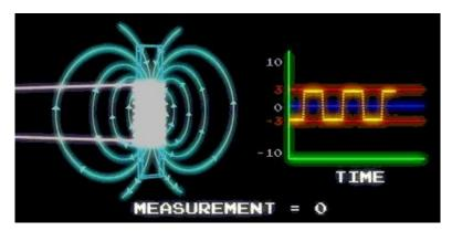
Figure 12: Measurement by changing the direction of the electric current without an external magnetic field
