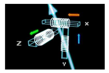
Figure 14: 3D-Measuring with three Fluxgate magentometers [13]
