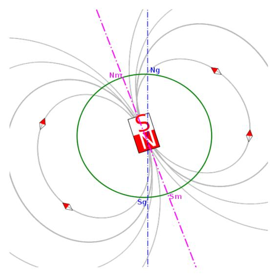
Figure 1: The Earth's magnetic field approximated by a bar magnet
